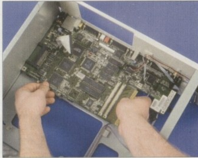
After removing your A1200's motherboard it is transferred to the Tower case and screwed into place. Notice the adapter (right hand) plugged into the A1200's trapdoor expansion connector. This connects the busboard to the A1200 motherboard
